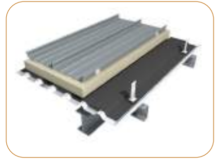
DOUBLE SKIN ROOFING
